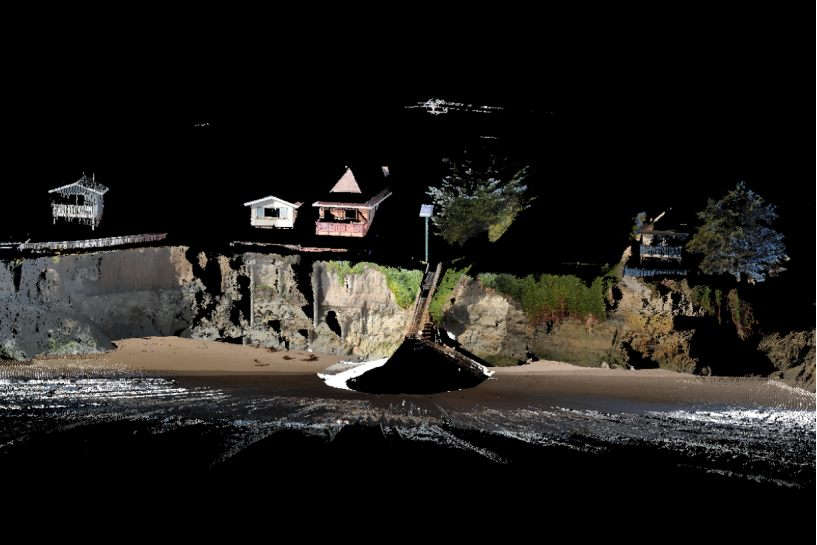
Different LiDAR scans over time allow the rates of erosion and other changes to be measured in Isla Vista.
